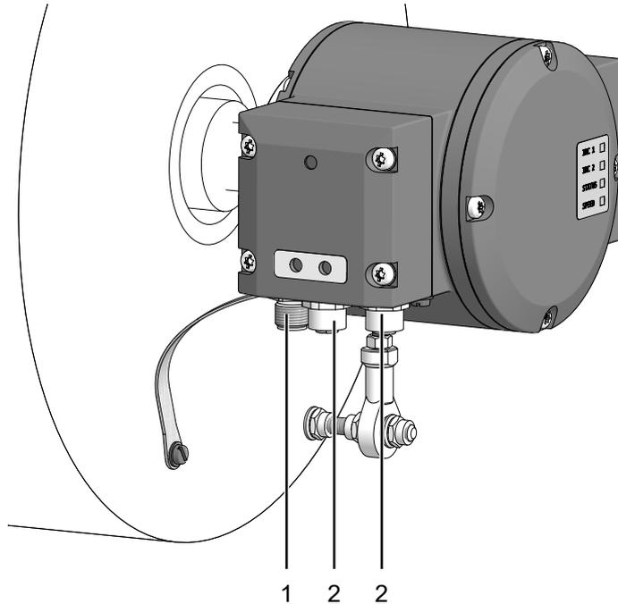
Abb. 4: Anschlüsse HMG10 EtherCAT
