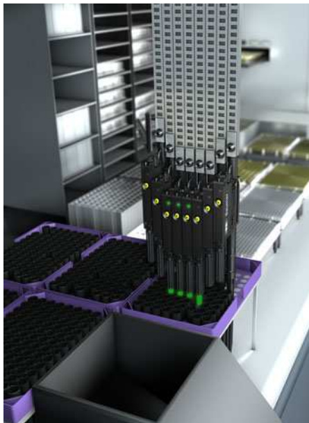
Figure 2: Detection of small pipette tips in the laboratory with ultrasonic sensors
