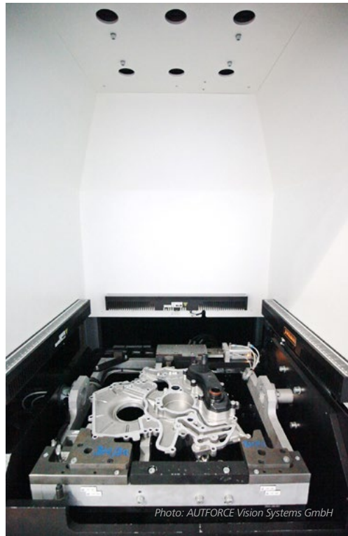
The illumination dome provides optimum conditions for surface metrology to filter traces of machining the component surface.
