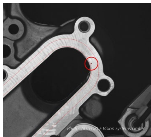
Reliable detection of blowholes from 0.4 mm upward at components sized 350 x 400 mm, with logging of position and size.
